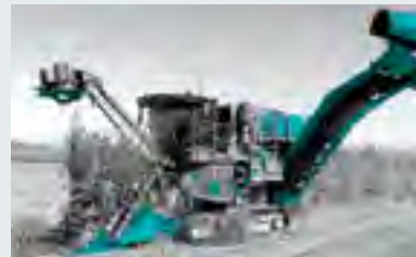
Keeping machinery clean – Pictured: Key sterilisation points for RSD on harvesters indicated in Blue.
