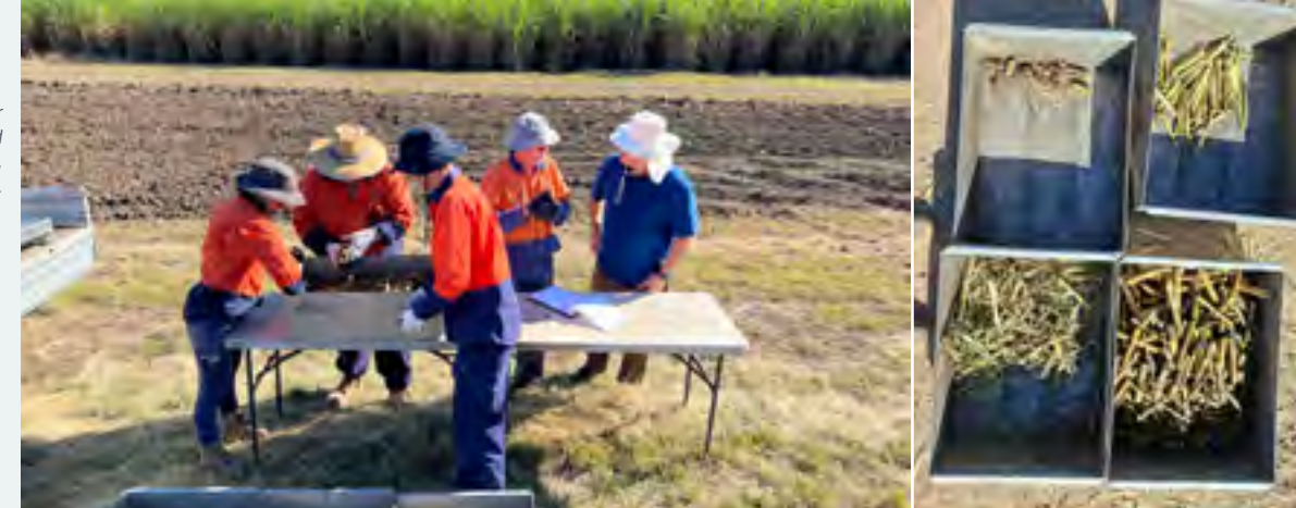
Pictured (left and right): During trials, for each test fan speed, a sample was collected from the bins and sorted into billets, tops, trash and cane roots.
