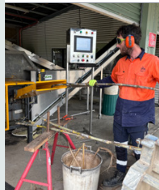
Pictured above: Whole stalk CCS samples cut from a family plot are fibred for assessment by SRA's SpectraCane™ unit. Each sample is barcoded to trace the sample (and its data) from its trial plot to the lab and finally captured and stored instantly in SRA's plant breeding database, SPIDNet.
