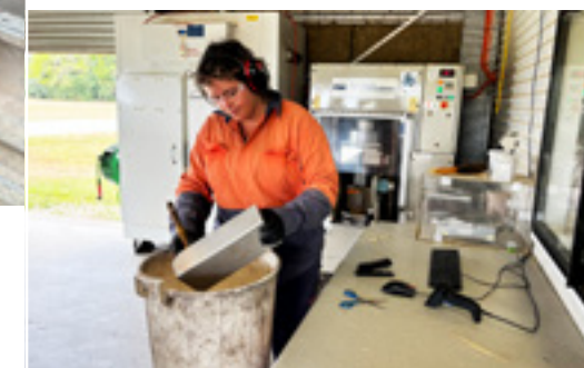
Pictured above left and above right: Juice from every tenth sample is then extracted using a hydraulic press (above left). Juice samples are processed through the wet-lab to measure Brix and Pol (above right). The Brix, Pol and fibre content from these 1 in 10 samples are then used to validate the NIR data to ensure accurate CCS data is collected and used.
