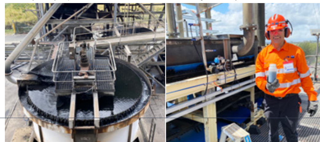
Elements in a boiler fly ash management system typically include: (left) an ash clarifier, seen from the top, and (right) an underflow belt filter, pictured with QUT Senior Research Fellow and Senior Engineer, Anthony Mann.
