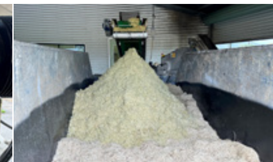
Pictured above left and above right: Fibred sample from each plot (pictured above left) being scanned using Near Infrared (NIR) to predict sugar content (CCS) and fibre content (% fibre). Once scanned by SpectraCane™ fibre from every tenth CCS sample is kept for validation purposes, while the rest is disposed of (pictured above right).
