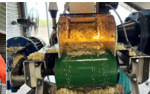
Pictured above left and above right: Fibred sample from each plot (pictured above left) being scanned using Near Infrared (NIR) to predict sugar content (CCS) and fibre content (% fibre). Once scanned by SpectraCane™ fibre from every tenth CCS sample is kept for validation purposes, while the rest is disposed of (pictured above right).
