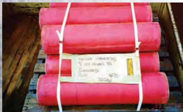
Figure14: Rubber coated harvester feed rollers improve the quality of billets for planting.
