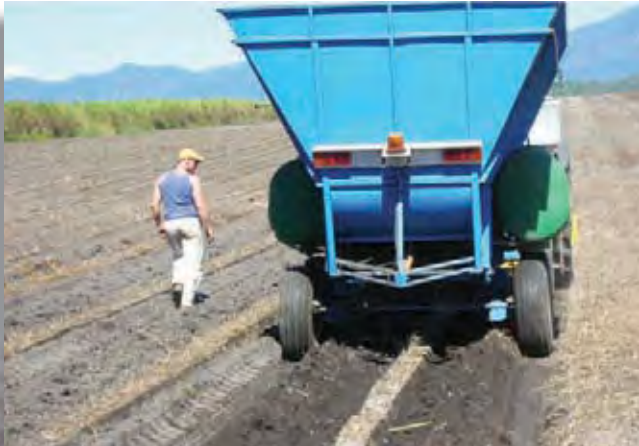
Figure10: Planting cane directly into soybean stubble with no prior cultivation. Undisturbed stubble on right.
