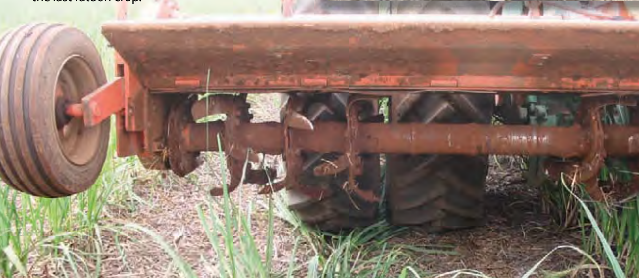
Figure 9: Rotary hoe modified for zonal tillage in the last ratoon crop.
