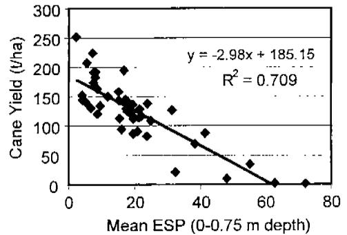
Fig. 2—Relationship between cane yield and soil sodicity (exchangeable sodium percentage, ESP) in the 0–0.75 m depth layer.
