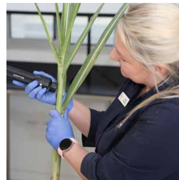
SRA Manager Industry Services Operations Heidi du Clou using a MicroNIR tool to demonstrate how the light source interacts with the surface of material.
