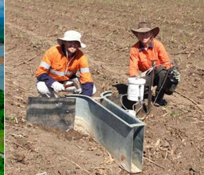
BBIFMAC's Angus Houston and Arwen Rickert install a San Dimas flume and water height logger.
