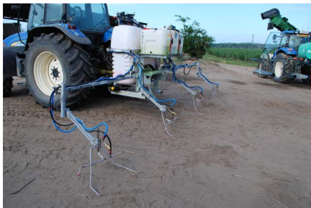
Above: DAF dual circuit sprayer – image on the right demonstrates two different circuits in operation using dye in the side nozzle circuit.
