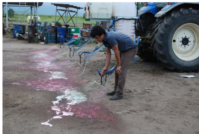
Above: DAF dual circuit sprayer – image on the right demonstrates two different circuits in operation using dye in the side nozzle circuit.
