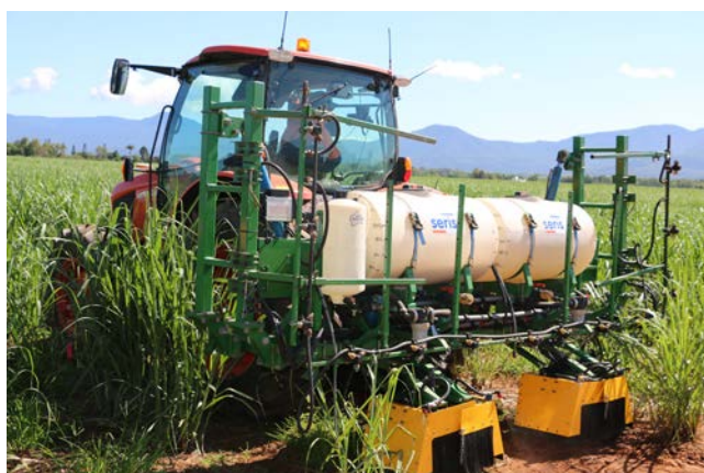
Above: Spray hood system utilising two spray circuits.
