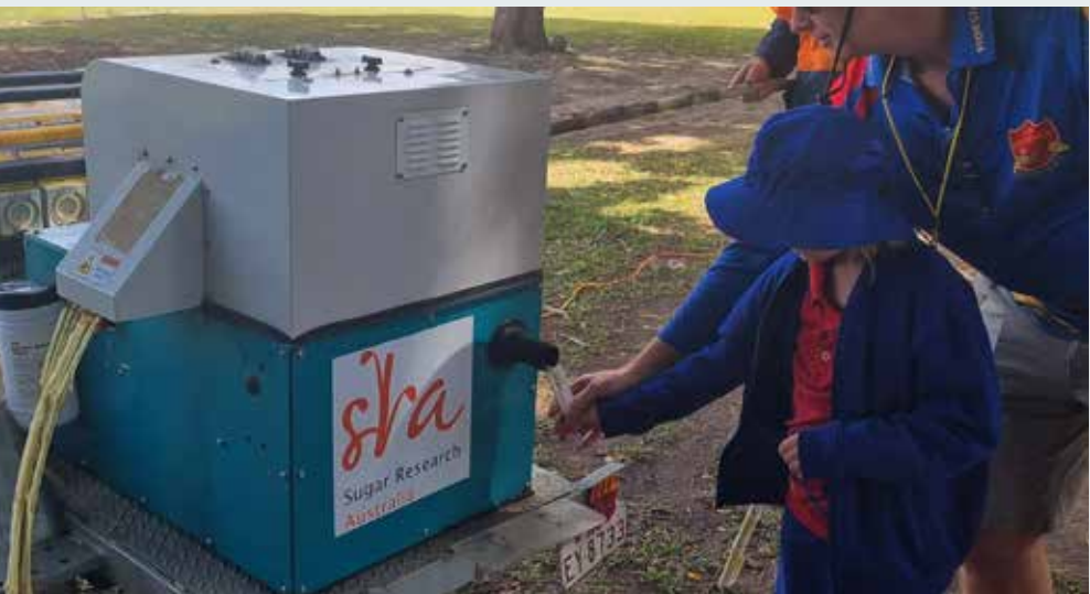
(Left) To test the sugar content of a stool of cane: Step 1: Run it through SRA's mobile maturity trailer and Step 2: take your juice sample. (Below Left) Step 3: Add your cane juice sample to the digital refractometer. (Below Right) Step 4: Take your reading.
