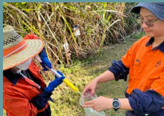
eDNA samples are bagged and sent to the laboratory for extraction and identification by DNA sequencing. Work on DNA extraction and rapid testing in the field is progressing in parallel with simple sampling methods.
