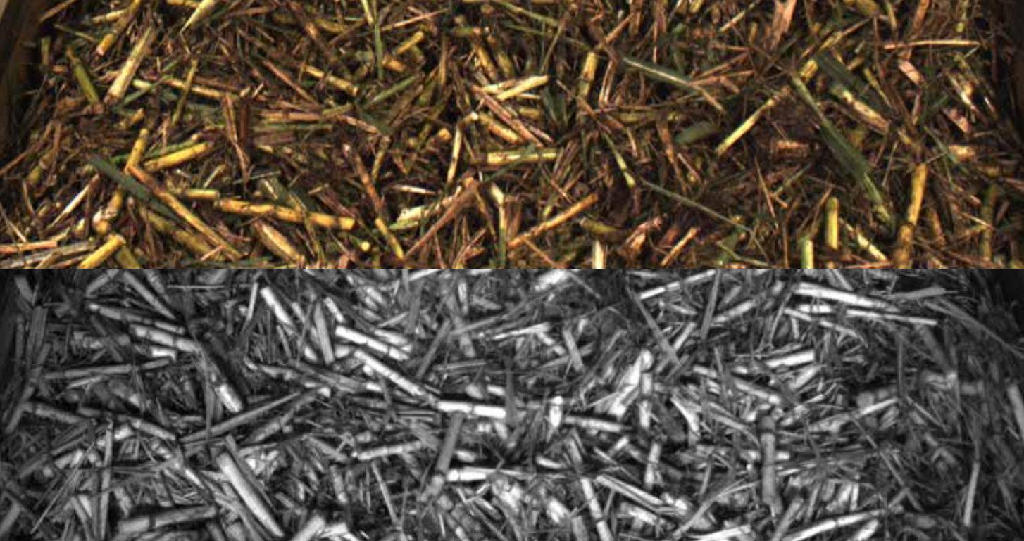
(Above) RGB colour image of cane billets coming into Tully Sugar Mill. (Below) NIR image of cane billets.
