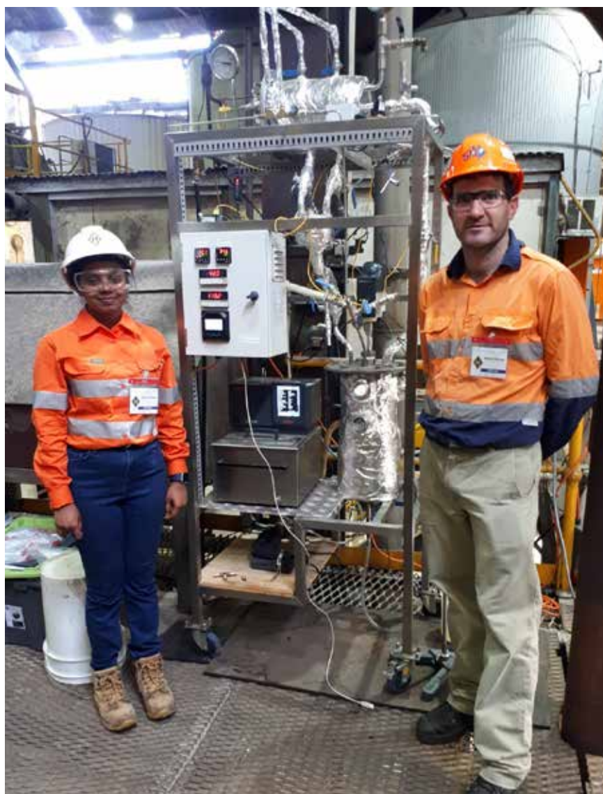
PhD student Chalani Marasinghege and QUT's Darryn Rackemann monitor operation of the pilot evaporator rig at Rocky Point Mill.
