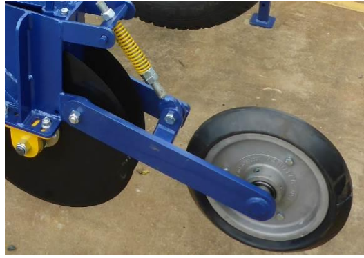
Figure 1. Press-wheel assembly (behind a double-disk opener in this picture). Credit : Hodge Industries.
