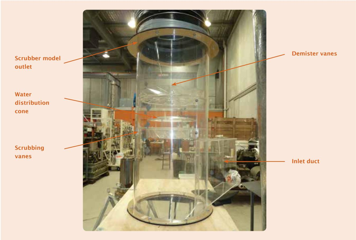
Above: Wet scrubber scale model used for CFD validation measurements.
