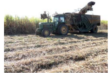
Measuring cane yield with commercial harvesters and weighing equipment. Sucrose and fibre content are analysed by Near Infrared Spectroscopy (NIR).
