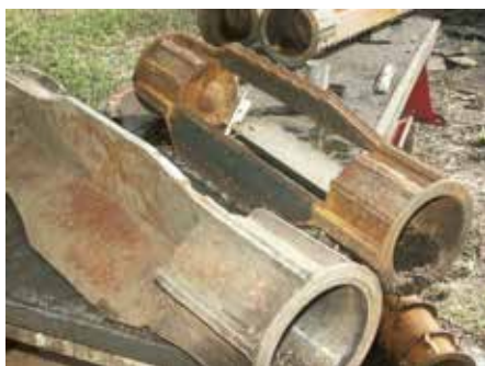
Above: Butt-lifter (solid) and open butt-lifter out of the harvester
