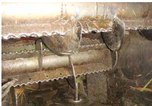
Above: Spiral wound knockdown roller and standard finned roller.
