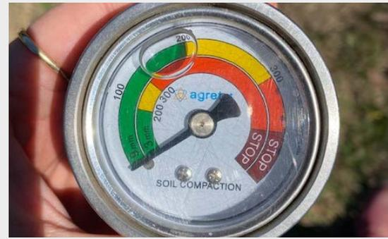
Figure 2: The face of a penetrometer pressure gauge.
