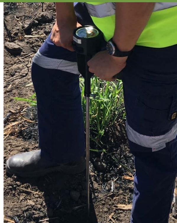
Figure 1: Penetrometers are a simple way of measuring whether compaction is a soil health constraint.
