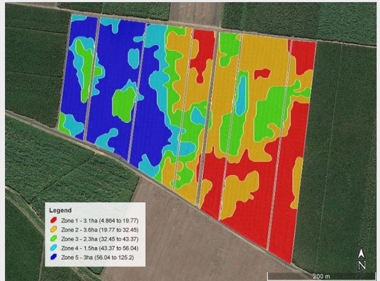
Figure 2. Typical EC map generated by TSM unit. Note the wide variation in EC<sub>a</sub> from 5 to 125 dS/cm
