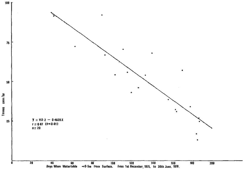
Fig. 7—The relationship between yield and number of days when water-table was less than 0.5 m from the surface.
