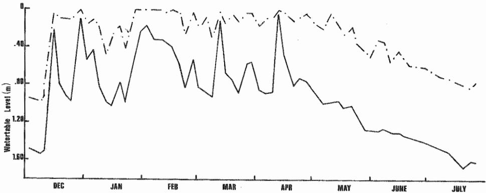
Fig. 3—Bi-weekly readings of water-table levels—site 3.
