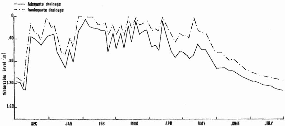
Fig. 4—Bi-weekly readings of water-table levels—site 4.
