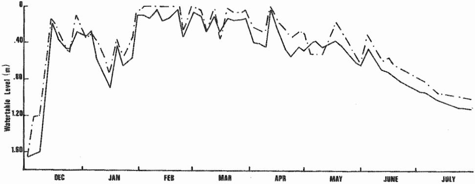
Fig. 2—Bi-weekly readings of water-table levels—site 1.
