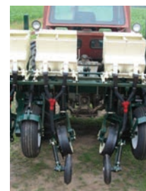
Images 5 and 6: Variations of the two types of press wheels.
