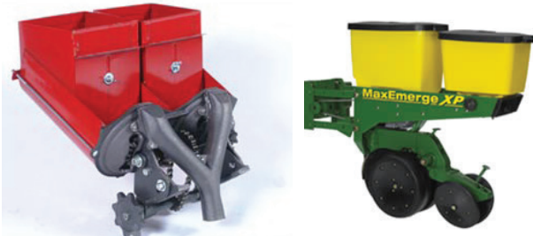
Image 2: Inclined plate type seeder.
