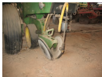
Images 5 and 6: Variations of the two types of press wheels.
