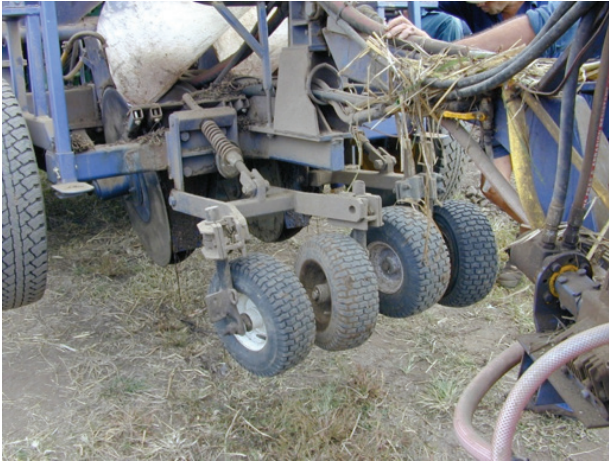
Above: Twin inclined press wheels on a cane planter that press each side of the sett. Pressure can be set by the spring adjustment.
