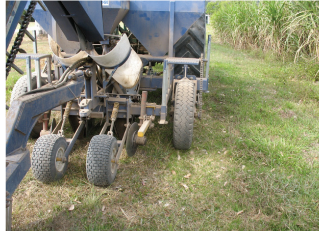
Above: Straight single wheels that press over the top of the sett.
