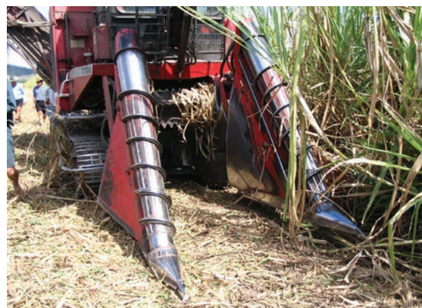
Image 3: Widened front for harvesting dual rows at 0.5 m – the throat width has been increased from 900 mm to 1050 mm.
