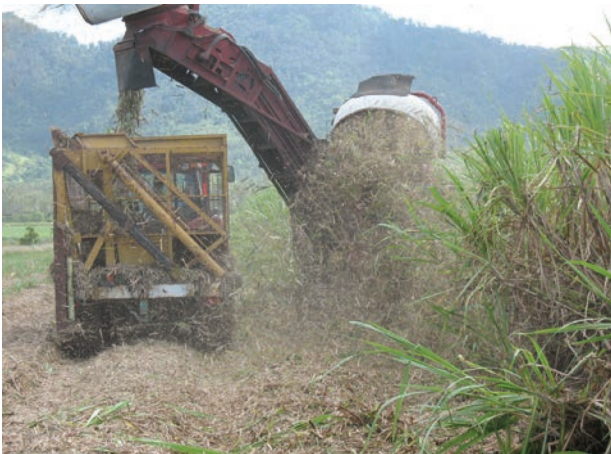
Image 4: Harvesting 2 m dual rows with an extended elevator allowing two rows between the harvester and the haulout. The elevator has a 900 mm extension over the standard length.
