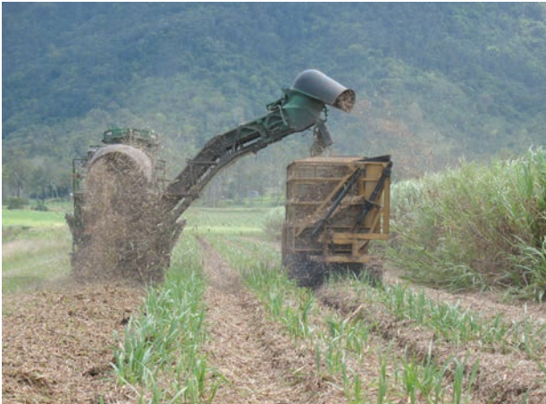
Image 4: Harvesting 2 m dual rows with an extended elevator allowing two rows between the harvester and the haulout. The elevator has a 900 mm extension over the standard length.
