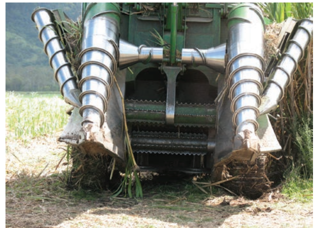
Image 6: Modified harvester front with 1300 mm wide throat and 780 mm wide base cutters and 2 m track centres.
