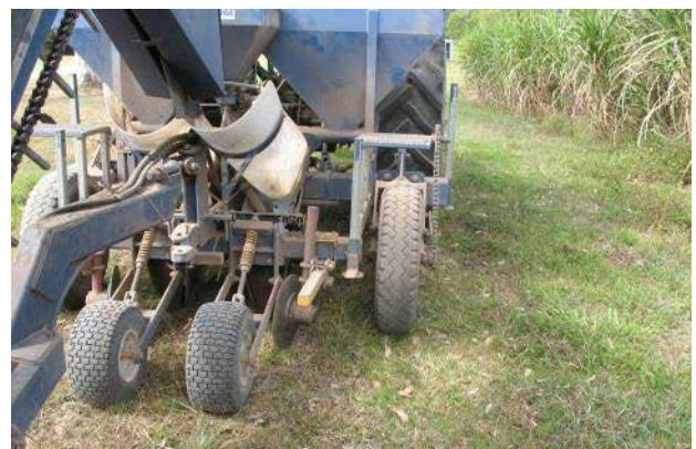
Image 7: Dual-row double-disc-opener planter.
