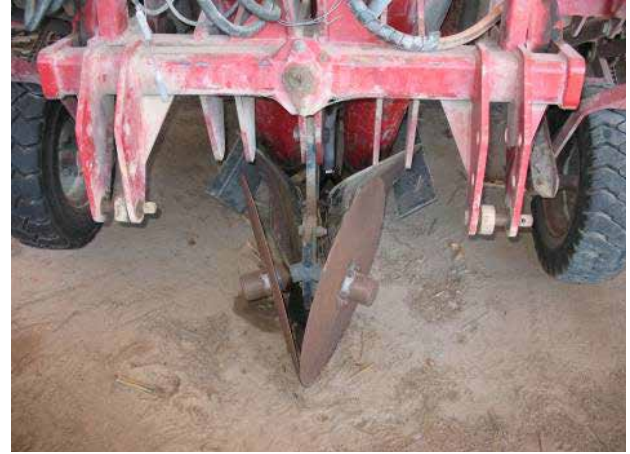
Image 10: A double-disc-opener setup on a wide-chute billet planter.
