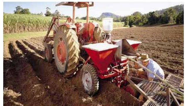
Image 1: Conventional whole-stick planter - note the deep planter furrow.
