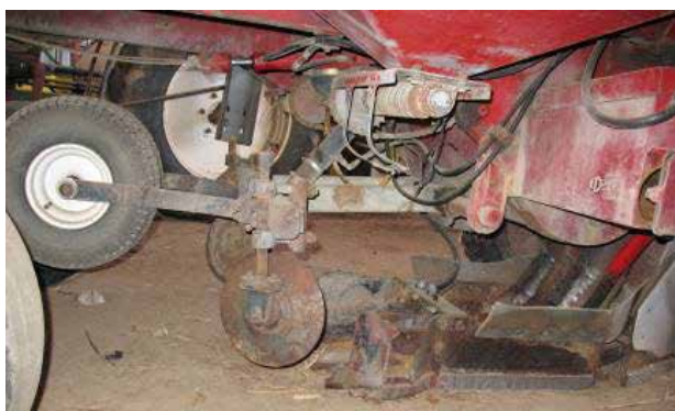
Image 2: 500-mm wide chute on a billet planter. Note the small covering disc.
