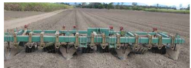
Image 9: Three-row light-disc bed former producing consistent, well-worked beds.
