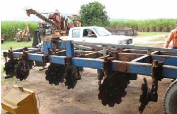
Image 5: Three-row, heavy-duty disc bed former.
