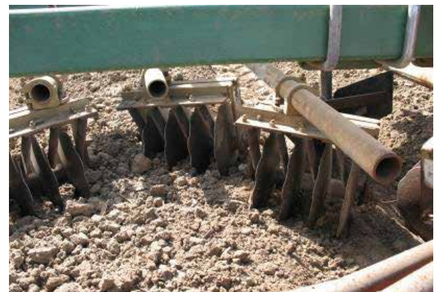
Image 8: Bed former with gangs of light discs forming the beds after the furrowing sweeps.
