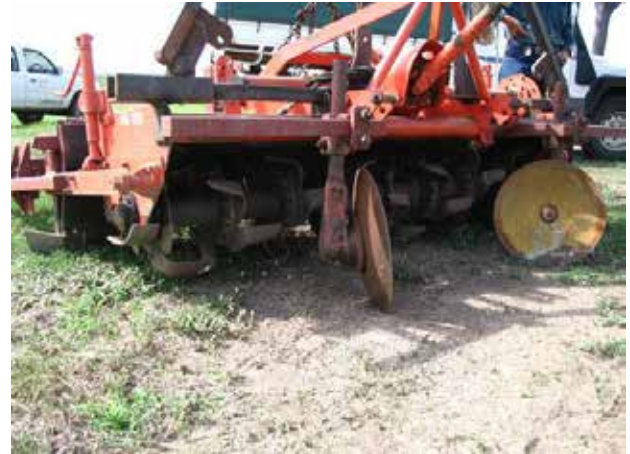
Image 11: Hill-up disc in front of the rotary hoe.
