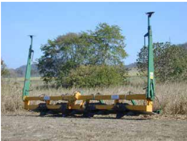
Image 2: Four-row plough-type bed former.
