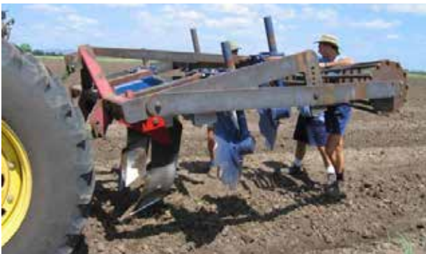
Image 6: Heavy-duty, disc bed former with a ripper to rip the beds.
