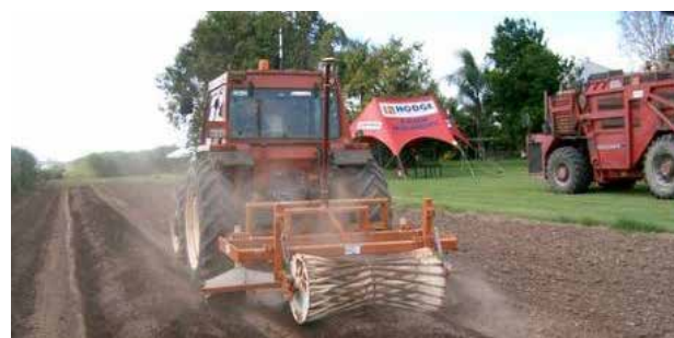
Image 1: Scraping-type bed former in operation. Note the rounded beds and the flat interspaces.
