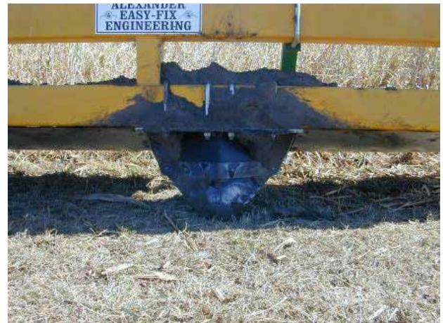
Image 3: Plough foot of a plough-type bed former.
