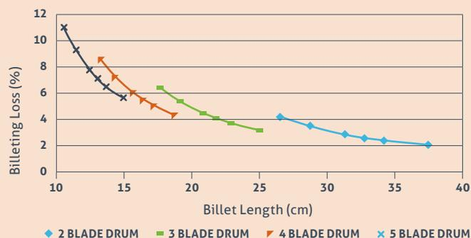
Billet length is also determined by feedtrain speed. Research has shown that the ratio of the surface speed of the feed rollers and the average blade speed is the most important driver of the amount of juice lost per cut. Loss per cut is optimised when this ratio is around 55-60% (optimised feedtrain). As this ratio gets below 50%:
