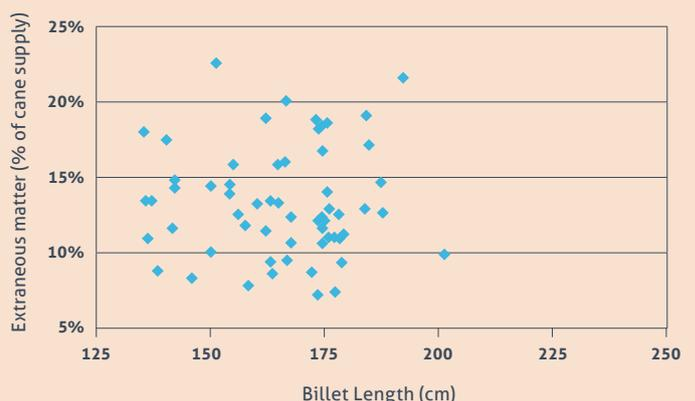
Cutting shorter billets increases billeting losses and increasing the number of chopper blades shortens the billet and increases losses as shown in the graph below.
