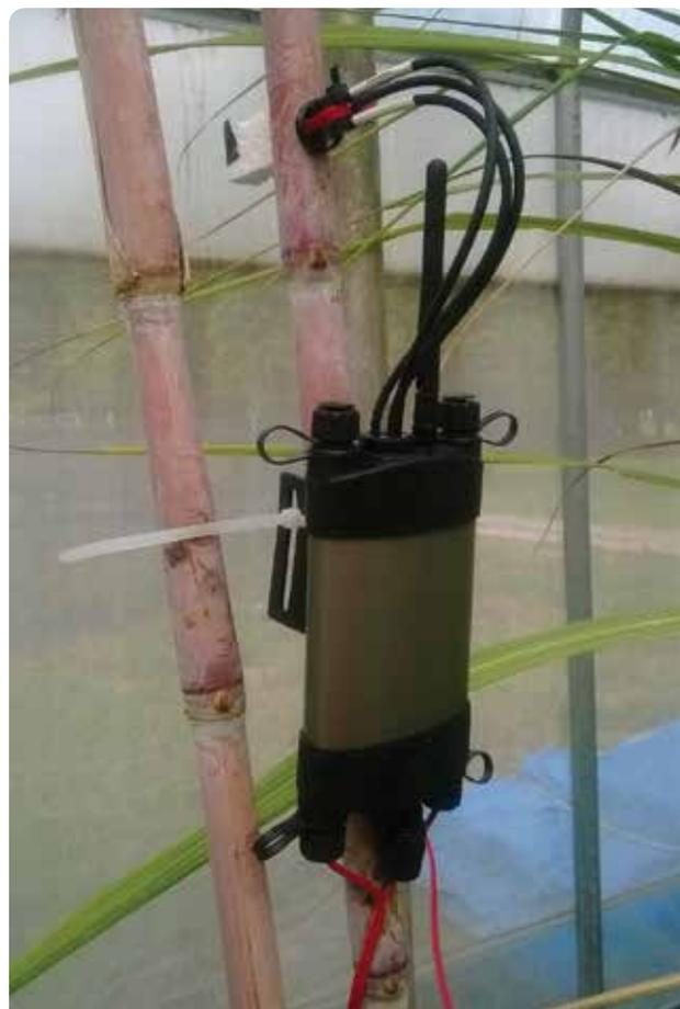
Sap flow meter connected to the sugarcane stem to record a real-time electrograph of sap flow in the stem.
