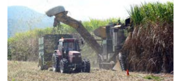
Measuring cane yield with commercial harvesters and weighing equipment. Sucrose content (CCS) is analysed by Near Infrared Spectroscopy (NIR).
