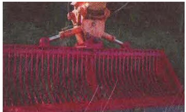
*Drain rake removes vegetative matter and leaves silt behind.*
