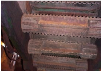
Commercial harvester – aggressive feed-train.
