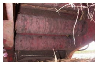
Modified harvester – rubberised rollers.
